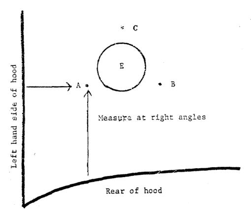
E is 3.50" diameter hole, center of which is 9.75" from left side of hood and 13.125" from back of hood
